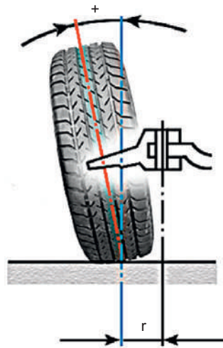
Figure 4.66 Positive camber ( r = scrub radius)
